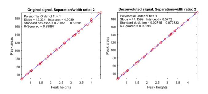
Test 3: More-overlapped peaks work better with deconvolution
