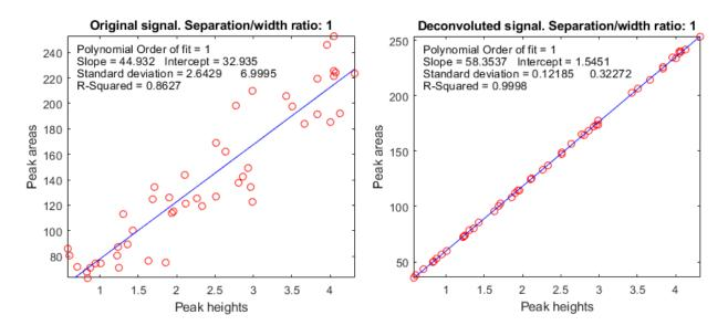
Test 11: When peaks merge into a blob with bumps: deconvolution method still works well.
