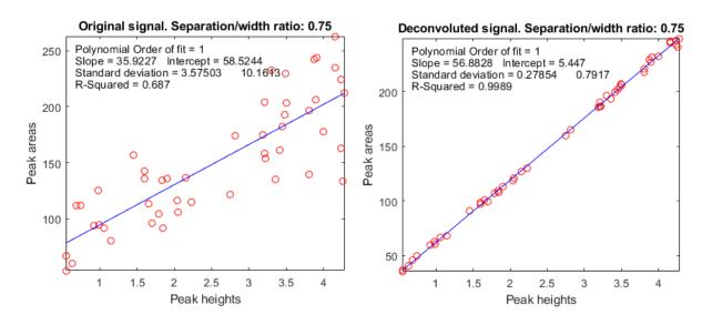
Test 12: If peaks fuse into one peak, even the deconvolution method performs poorly.
