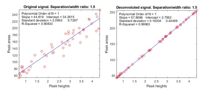
Test 9: Even closer spacing; deconvolution method still achieves baseline resolution
