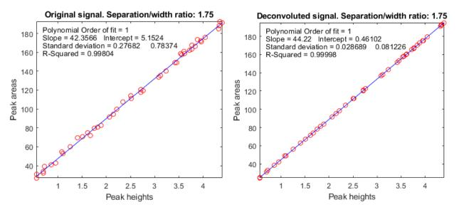
Test 4: Heavily-overlapped peaks work significantly better with deconvolution
