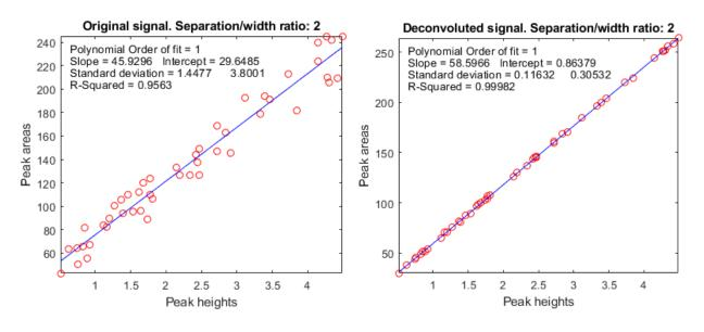
Test 8: Even closer spacing, deconvolution method achieves flat baseline between peaks.
