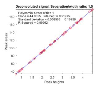
Test 5: Severely-merged peaks work far better with deconvolution
