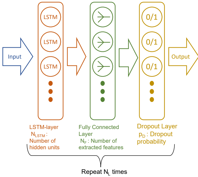
Figure 2: Architecture of the neural network utilized for ocean wave forecasting.
