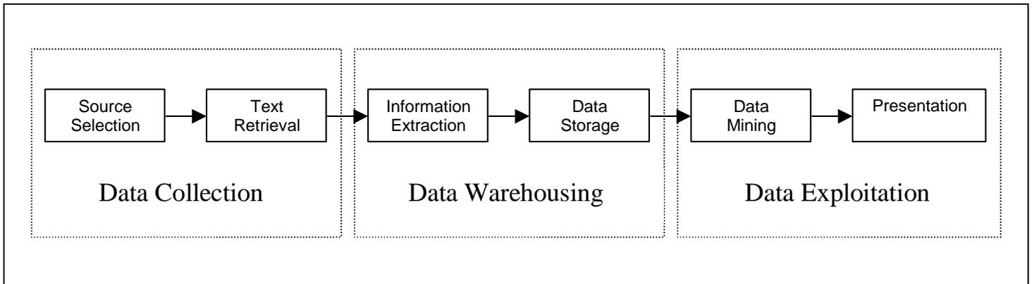
Figure 1. The textual data mining architecture.
