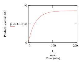
In a batch reactor, the enzyme eventually becomes completely deactivated, and there is no further conversion. The dynamic time constant for the product formation process is  $1/k_d$ . The eventual product level depends on the ratio of  $k_2$  and  $k_d$ , and is proportional to the initial amount of enzyme.
