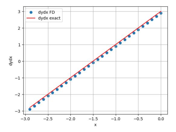
In conclusion, the FD approximation appears to be a relatively accurate approximation, but **Q:** What is the source of the small, constant difference between the curves?
