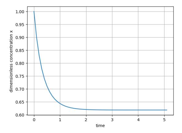
Note how the dimensionless concentration x approaches a steady state value of
