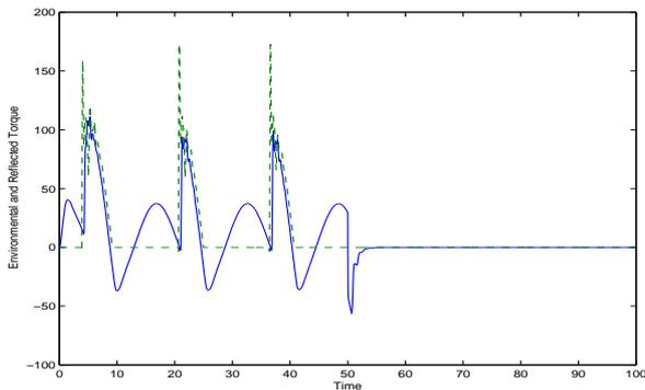
Figure 5: The reflected torque to the master  $F_m$  accurately tracks the environmental torque  $F_e$
