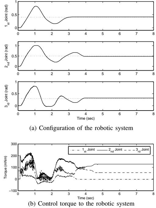
Fig. 9: Even when the derivative of time-varying delays is close to one, the stability and tracking performance are guaranteed by using the position feedback architecture.
