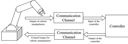
Fig. 1: The sketch of using communication networks to interconnect a robotic system with a controller.
