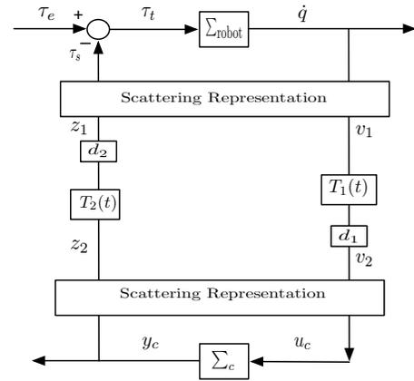
Fig. 4: The scattering transformation, together with the gains (dependent on the rate of change of delay) are used to ensure stability of the closed loop system.
