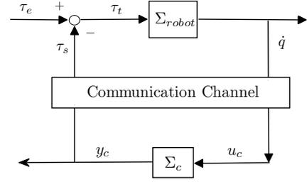
Fig. 2: A negative feedback interconnection of the robot dynamics and the controller.
