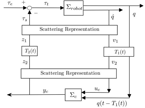
Fig. 5: A position feedback architecture with the use of scattering transformation is proposed to ensure the tracking performance and stability of the closed loop system.
