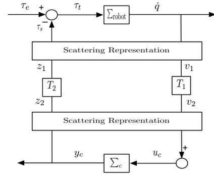
Fig. 3: A negative feedback interconnection of the robot dynamics and the controller with scattering representation.
