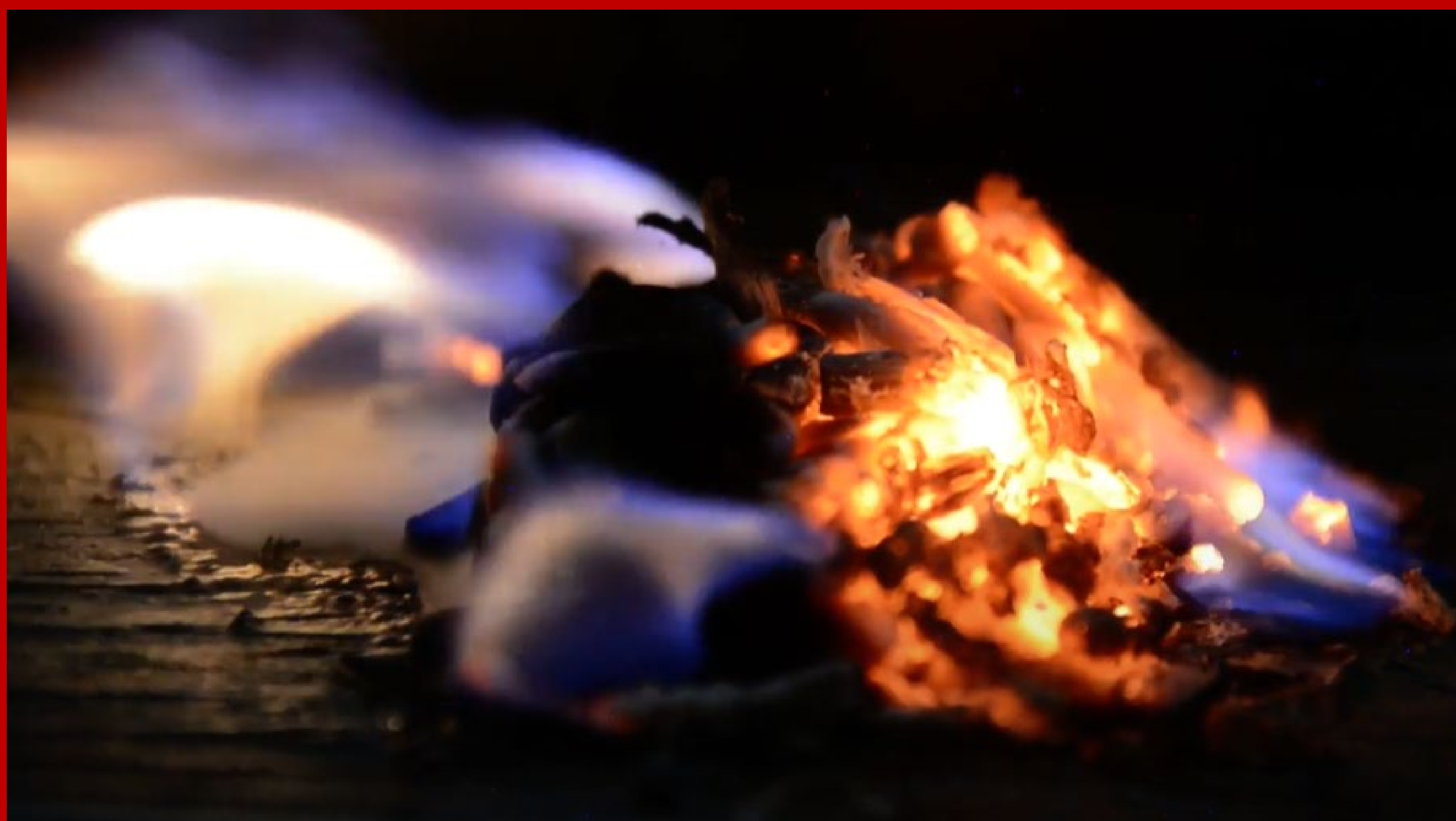
Figure 1: the firebrands on top of the wood sample in the wind tunnel
