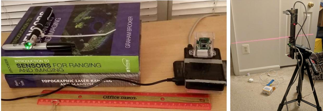
*Single beam laser bistatic configuration (left) vs. line laser bistatic configuration (right)*
