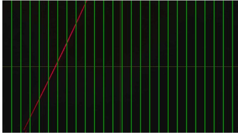
*Line laser orientation at the beginning of the alignment process (not currently aligned). Note the lack of parallelism between the red laser line and the green vertical alignment lines.*
