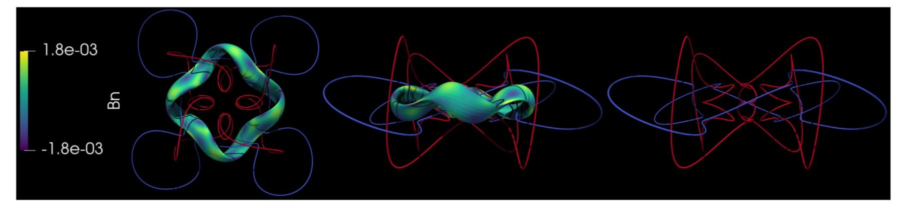
Three views of the helical coils with combined 24 + 29 = 53 meter length, generated from a voxel solution for the Landreman-Paul QH stellarator. The right-most panel only shows the coils for a better look at the geometry.
