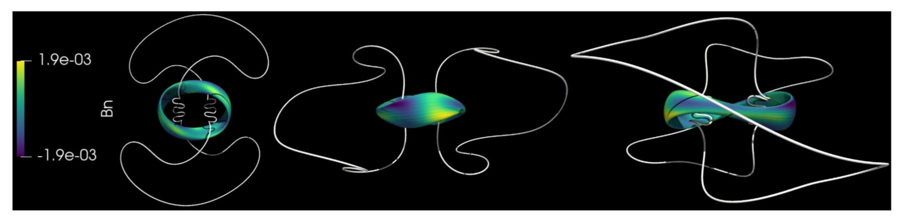
Three views of a 40 meter filament coil generated from a voxel solution for the Landreman-Paul QA stellarator.
