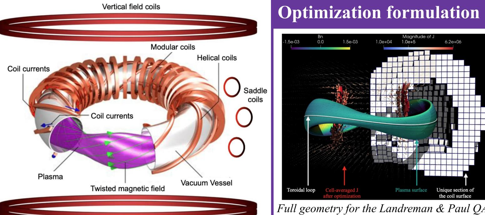
A classical stellarator, adapted from Proll (2014) and courtesy of C. Brandt. A combination of modular, *helical, saddle, and vertical field coils (red & orange)* are used to match a target  $\mathbf{B} \cdot \mathbf{n}$  at the plasma surface S.
