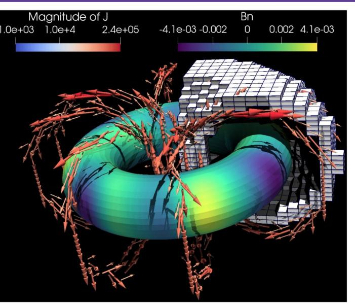
Full geometry & solution for an axisymmetric torus  $(\lambda > 0)$ . **B**•n errors are shown on the plasma surface S and the cell-averaged Jsolution vectors are color-coded by ||J||.
