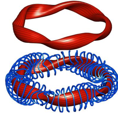
New approach: Directly optimize coil shapes for consistency with near-axis quasisymmetry. *A Giuliani et al, arXiv (2020)*
