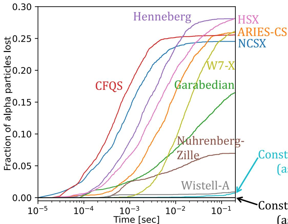
All configurations scaled to ARIES-CS minor radius (1.7m) and  $|B|$  (5.7 T)
