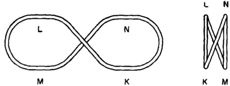
FIG. 2. Top and end views of a figure-eight stellarator.
