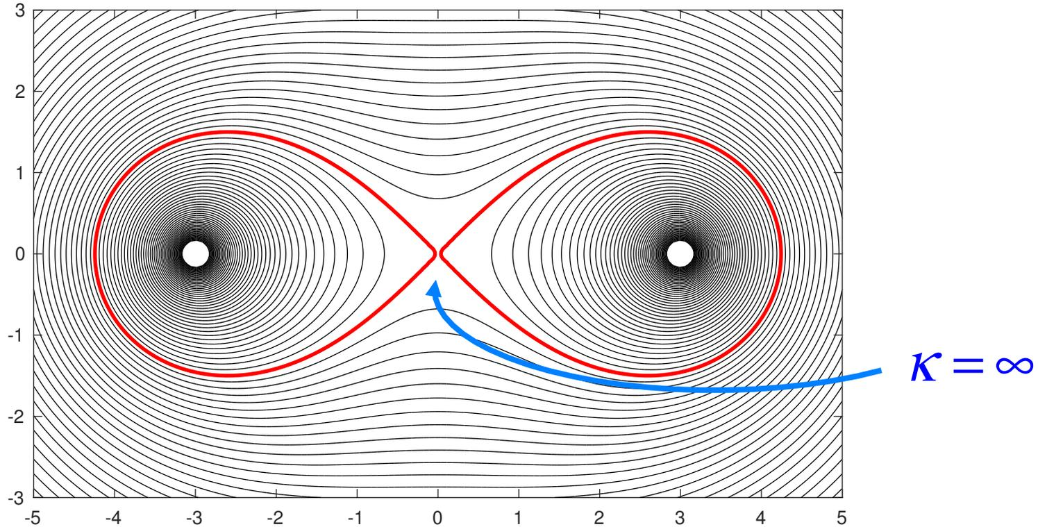
So a field line's radius of curvature is not a good measure of distance to coils.
