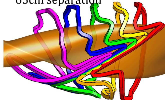
In a reactor, must fit  $\sim 1.5\text{m}$  “blanket” between plasma and coils to absorb neutrons
