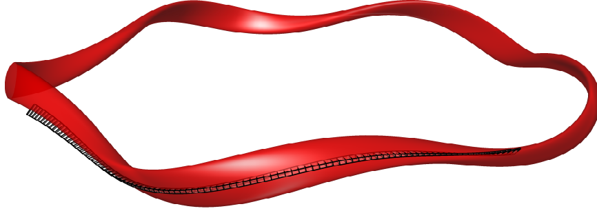
Figure 3.1: (Color online) 3D visualization of a flux tube domain in real space superimposed on a flux surface in the W7-X stellarator. (The perpendicular extent of the tube in was set for visualization purposes).
