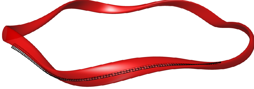
Figure 4.7: (Color online) 3D visualization of the \alpha = 0 flux tube domain in real space superimposed on the flux surface at x/a = 0.357 . (The extent of the tube in \psi, \alpha was set for visualization purposes). This is the same flux tube from Figure 4.6, but shown from \theta = [-0.73, 0.73] , where \nabla\psi \cdot \nabla\alpha = 0 and the ends of the tube have a rectangular perpendicular cross section.
