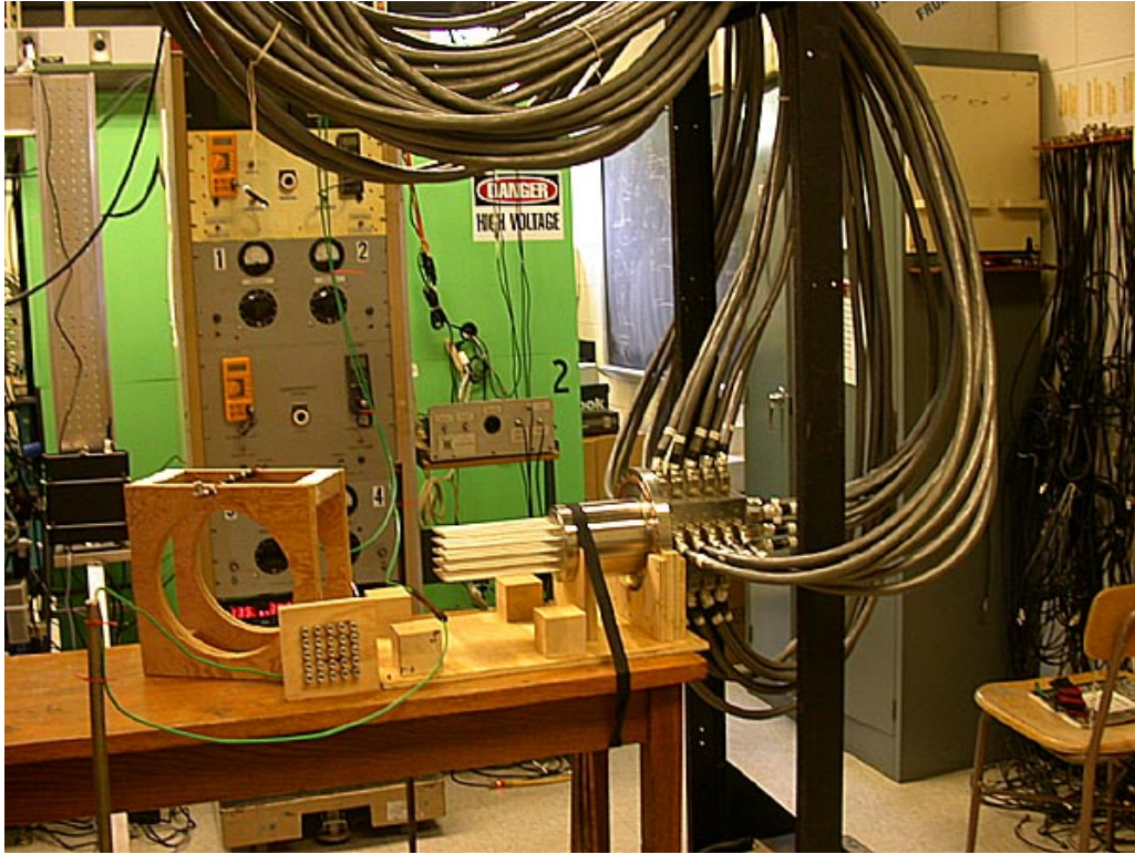
Figure D.2: The apparatus used for these vacuum field measurements. On the table are the Helmholtz coil, the “squasher” (see Figure D.6), and the “quasi-infinite” wire. The probe is not set up to measure any particular field at this point.
