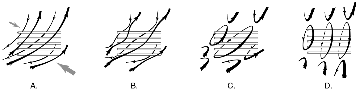
Figure 4.29: Possible mechanism for creation of the “roll” in a full-merging shot, as seen from a side view (looking +z ). A: Spheromak fieldlines come in from either side (cf. Figure 4.6.D) B: The stainless steel probe tines - which are more resistive than the copper but still somewhat conductive - slightly slow the incoming plasma near the probe. C: Consequently, reconnection occurs initially just outside the probe region, leaving reconnected rings of \mathbf{B} around the stalks. D: The rings equilibrate to form the roll.
