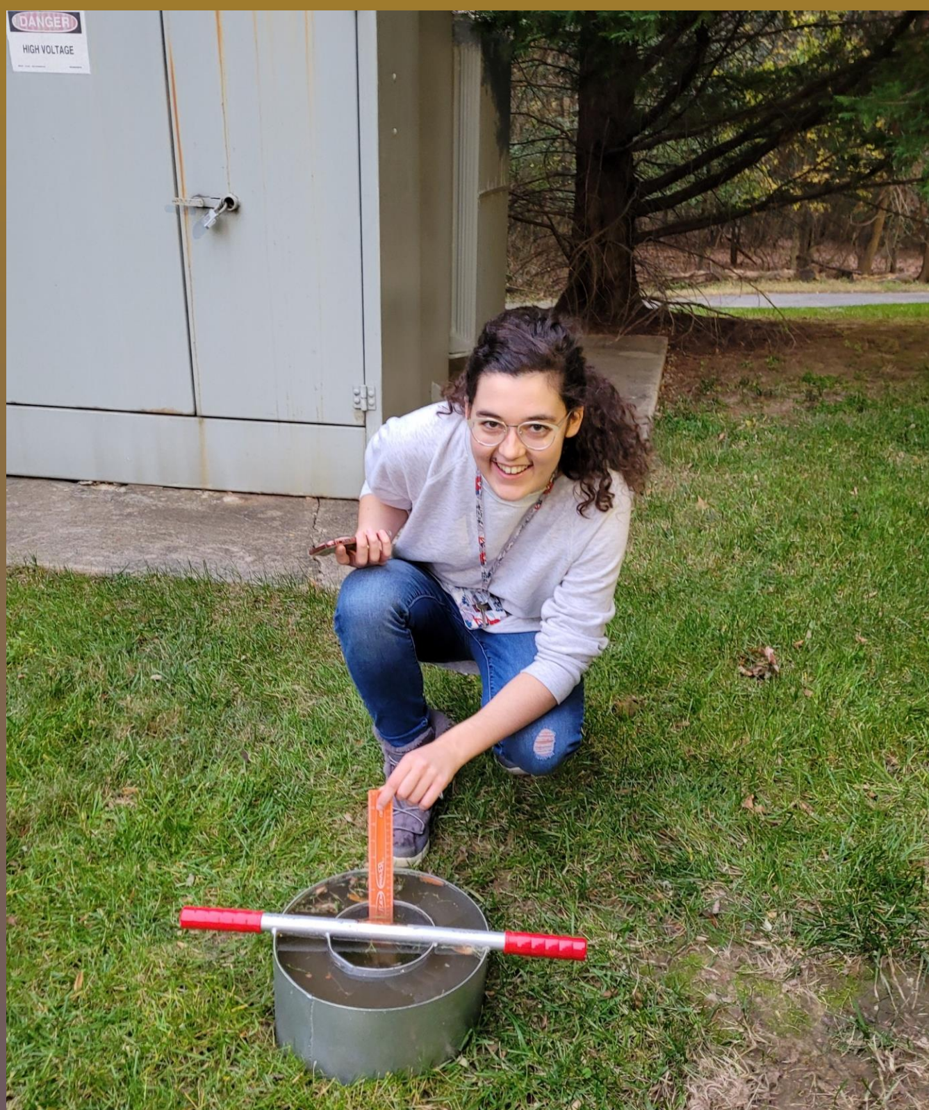
Conducting Average Water Infiltration Test
