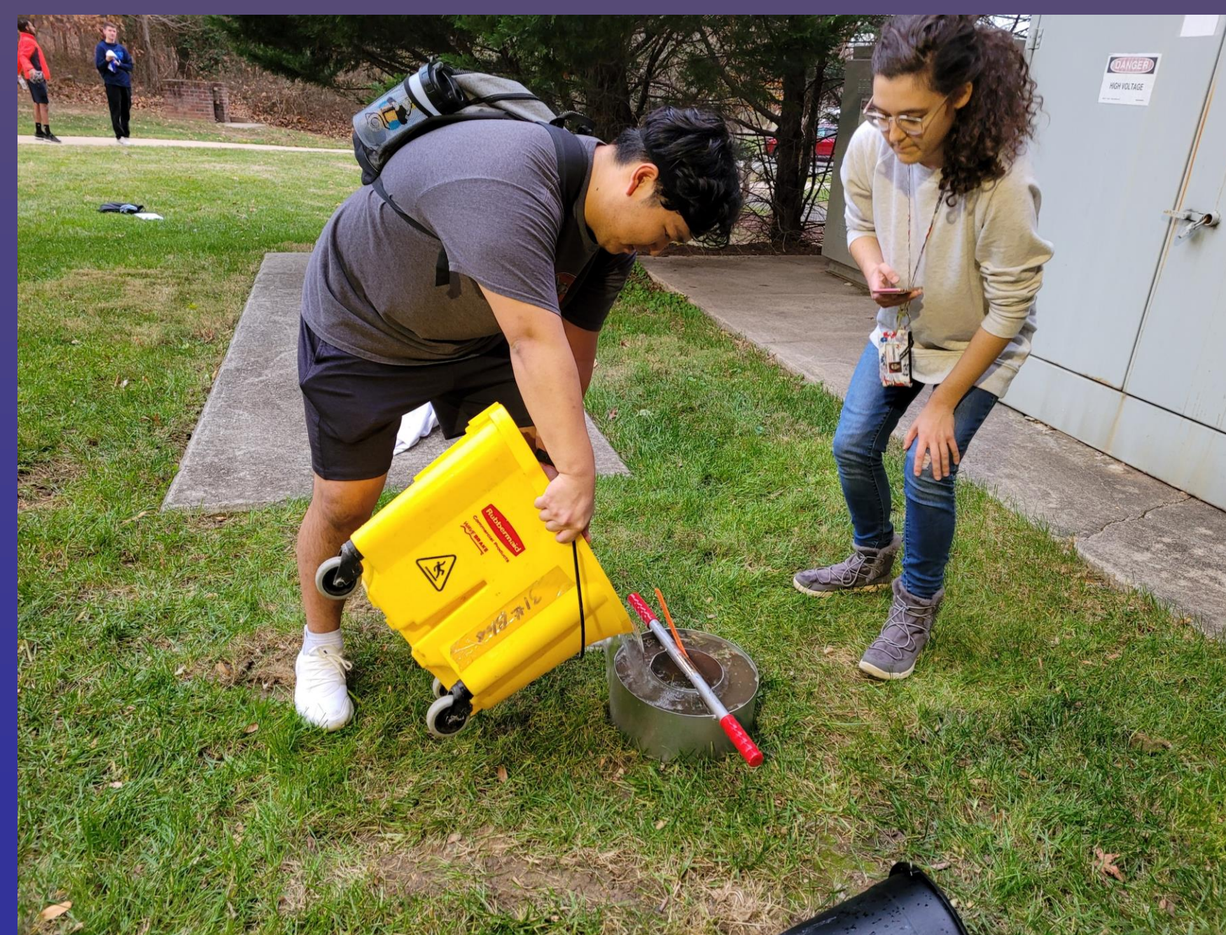
Conducting Average Water Infiltration Test
