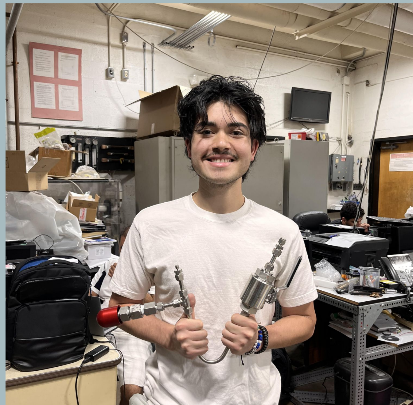
Showcasing the microreactor I built for small batch testing in hydrothermal liquefaction processes
