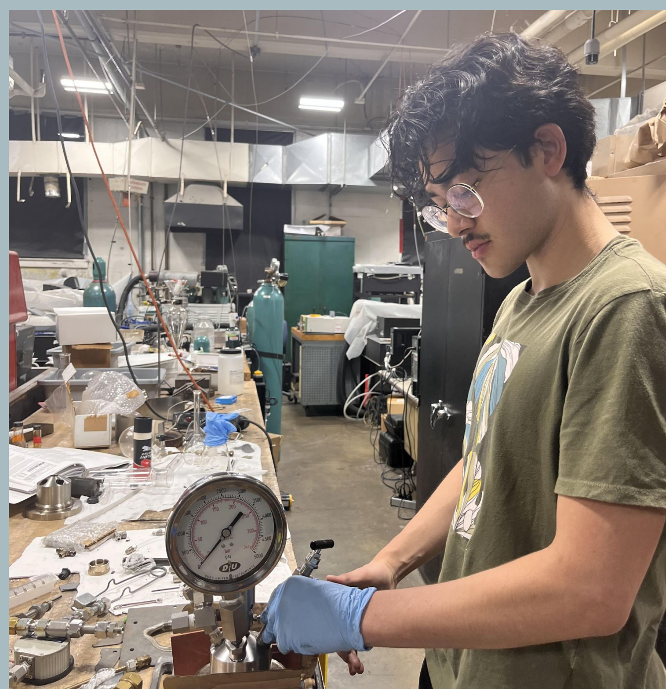
Working on a reactor vessel cover so that we can add a rupture valve to it
