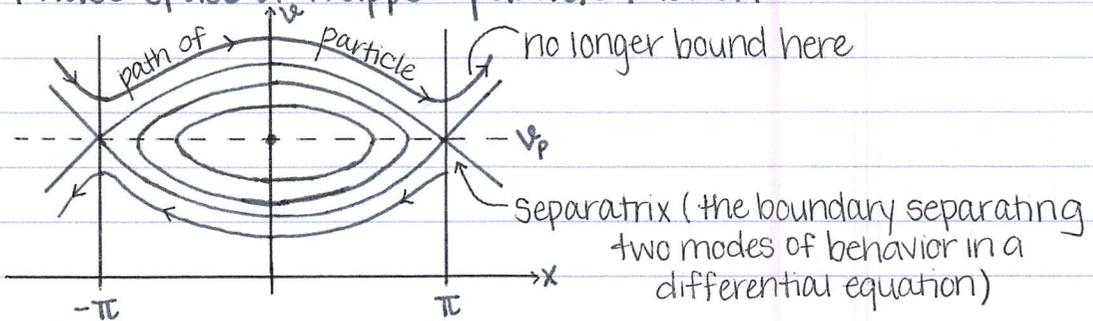
critical points — critical energy value beyond which the particle is no longer trapped
