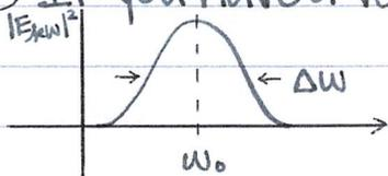
Here,  $\Delta\omega \gg \omega_b \rightarrow$  the particle sees many waves and sees coherent acceleration only for a short time
