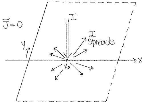
$\nabla \cdot \vec{J} = 0 \rightarrow$  the current density at any point  $\vec{x}$  is independent of time. Charges are in motion, however, there are a large number of charges executing the same amount of charge is passing through any fixed surface.
