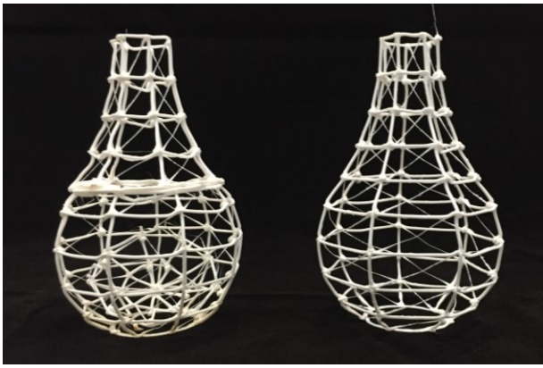
Figure 17: The same vase created in CAD in a multi-step approach (left) versus a single-step approach (right) results different physical appearances. On the left, the top section of the sphere fell into the model during the cutting process.
