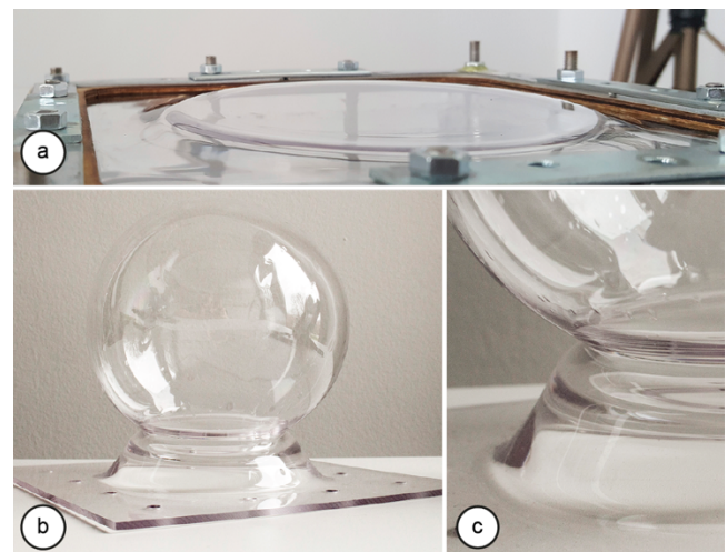
Figure 20: First steps of making a head sculpture with neck. (a) outline shape for neck, (b,c) adding the head.
