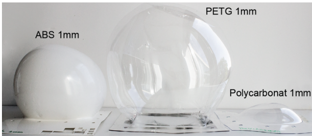
Figure 16: Results from our material stretch test.
