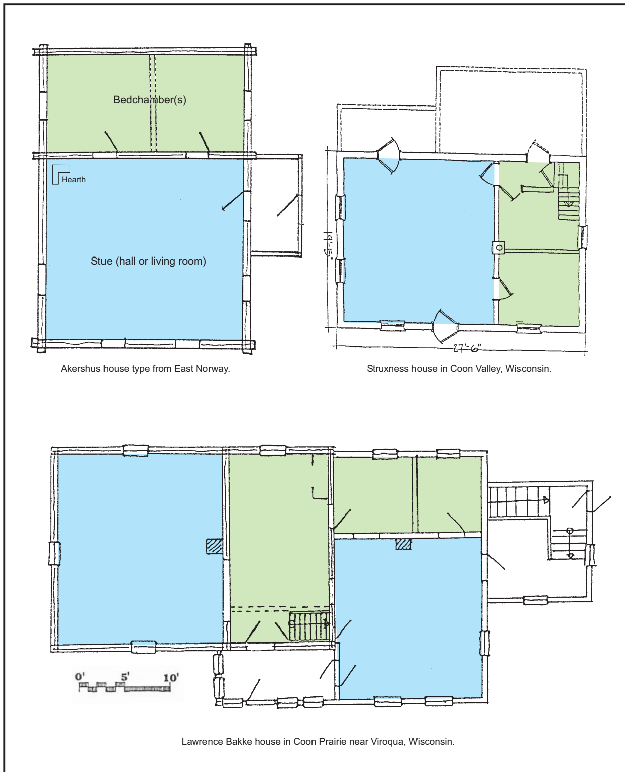
Figure 2.22. Floor plan of the Akershus house type and several examples of similar plans in Wisconsin (after Bakken 1994:77, 80).
