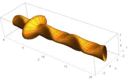
Fig. 5: This is a simplified 3D visualization of the beam. The bulge indicates altered shape in the injection line. The beam is squashed horizontally and vertically, alternating.
