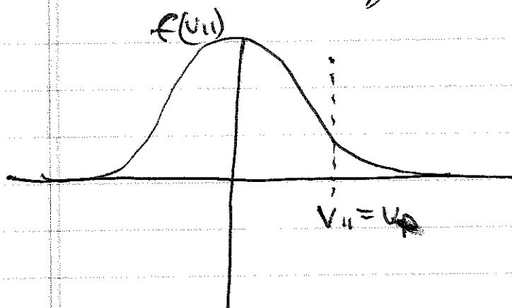
Damping occurs because particles with  $V_{||} \approx V_p$  see a nearly DC electric field. Particles slightly slower than the wave will gain energy from the wave while those slightly faster than the wave will slow down and give energy to the wave. More particles slower so wave damps.
