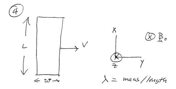
Since the wine is a pented conductor, the Emt must remain zeno so that I in the loop is finite. The magnetic flux cutting through the loop by Bo must be balanced by that due to the cumunt I.
