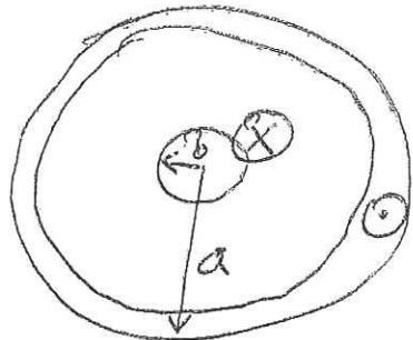
Calculate the inductance per unit length for currents going in the inner conductor and out the outer.
