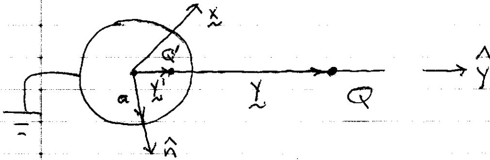
Zero potential on sphere  $\Rightarrow \phi(|x|=a) = 0$
