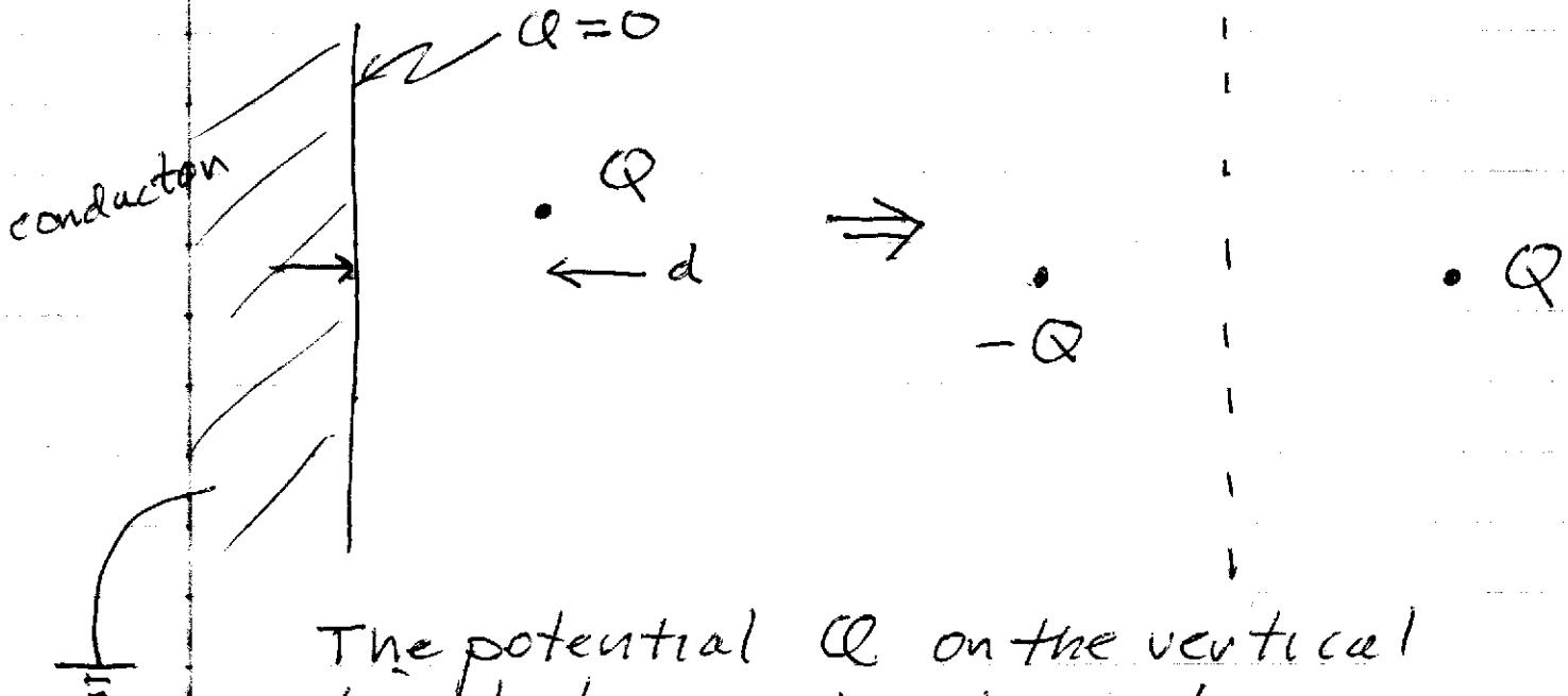
The potential  $\phi$  on the vertical line between the two charges yields the same BC's as the conducting plane. The potential on the right of the dashed line is the same as with plate. Why?
