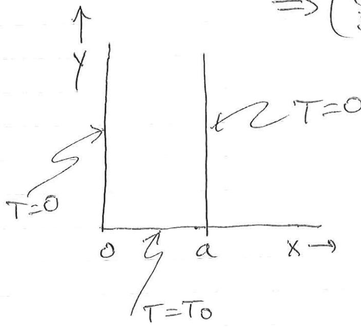
A rectangular system has a temperature  $T_0$  at a plate at  $y=0$  and zero temperature at the two sides. The system is open at the top
