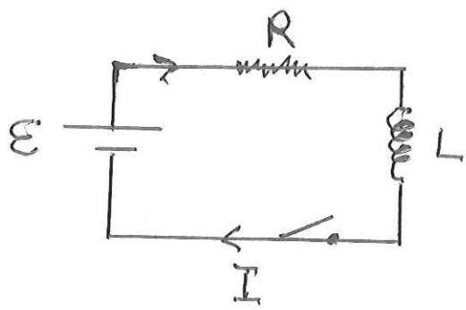
Consider an inductor  $L$  and resistor  $R$  in a circuit.
