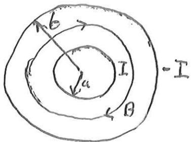
A co-axial cable has a current  $I$  flowing into the page (assume current on surface) ~~out~~ on the inner conductor and a current  $-I$  flowing out of the page on the outer conductor.
