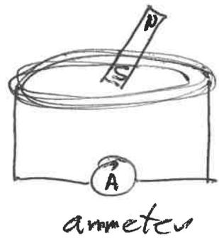
Move a bar magnet toward the coil  $\Rightarrow$  measure a current in the coil
