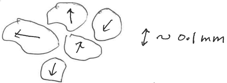
⇒ in an external field the domains align to produce very strong magnetic fields
