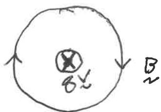
Right hand rule gives direction of  $\vec{B}$ : thumb along current and fingers wrap around to give  $\vec{B}$ .
