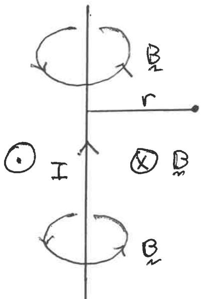
$$B = \frac{\mu_0 I}{2\pi r} \Rightarrow \text{infinite wire}$$
