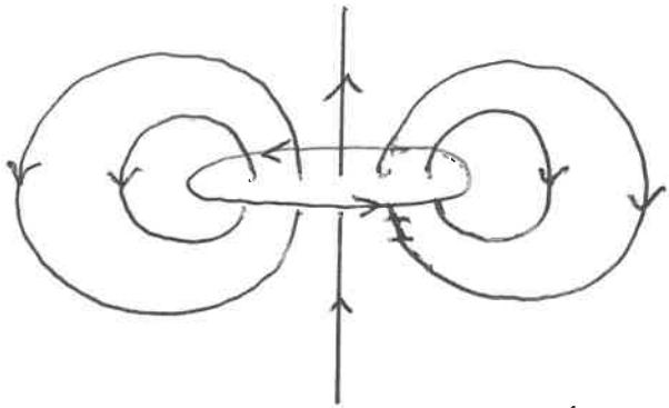
Close to the wire  $B$  are small loops around the wire  $\Rightarrow$  circles
