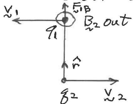
$$B_2 = \frac{B_2 v_2}{r^2} \frac{\mu_0}{4\pi} = \text{magnetic field from } B_2 \text{ at location of } q_1$$
