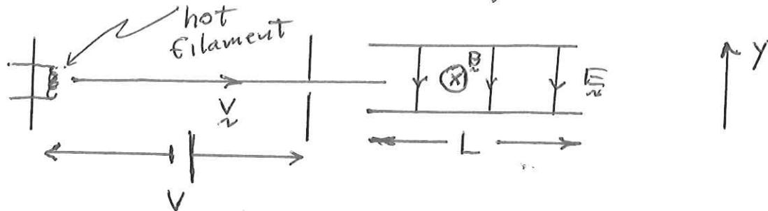
The hot filament produces electrons that are accelerated across the potential  $V$ .
