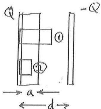
The dielectric has a width  $a$  that is smaller than the plate separation  $d$ .
