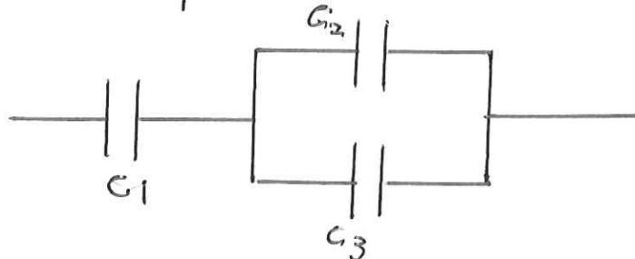
$C_2$  and  $C_3$  are in parallel  $\Rightarrow$  replace by single capacitor
