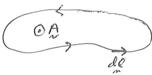
The top equation relates  $\underline{E}$  along  $d\underline{l}$  to  $\underline{B}$  perpendicular to  $d\underline{l}$  along  $d\underline{A}$ .
