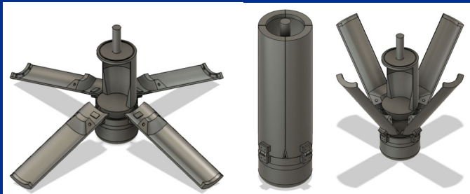
An image of our prototype drop assembly mechanism design in various stages of deployment, as shown from left to right: fully deployed, undeployed for storage or transportation, and partially deployed.
