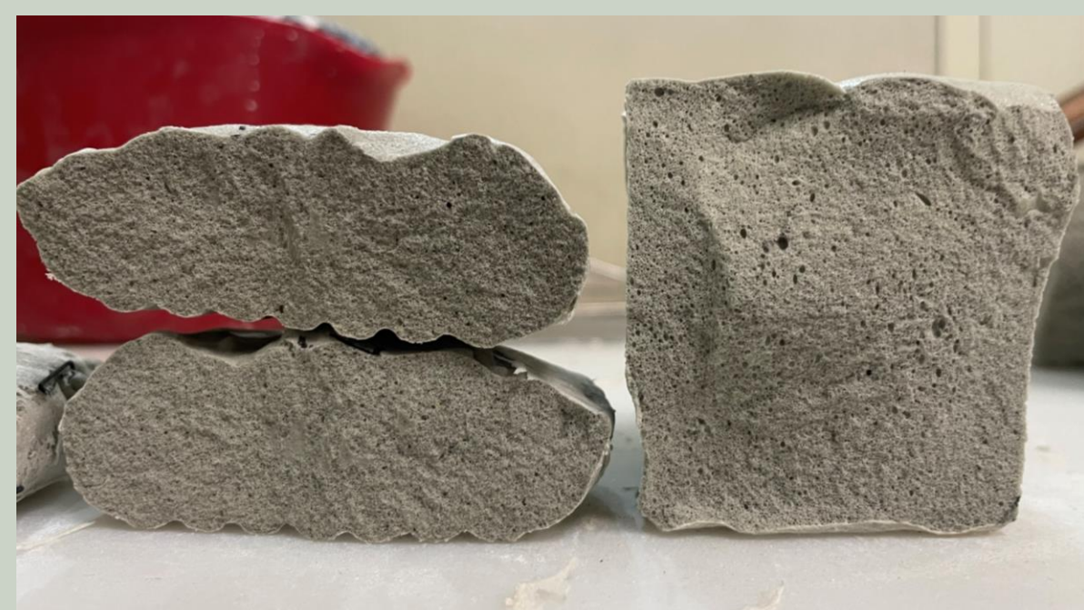
Figure 1 (top left): Lab produced FGA foam structure (left) compared to manufactured FGA foam structure (right).
