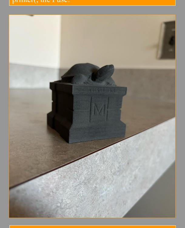
This testudo is a scanned replica of the real testudo statue printed on the SLS Fuse powder bed!
