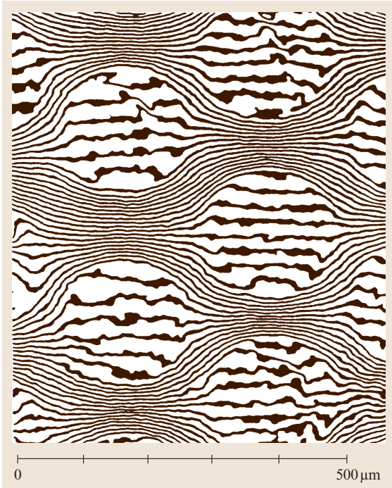
Fig. 22.18 Boron/aluminum composite subjected to a change of temperature of 110^{\circ}\text{C} . Microscopic moiré interferometry was used with f = 4800 lines/mm and \beta = 6 ; 35 nm/contour
