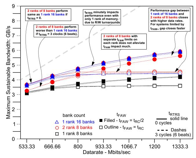
t<sub>RC</sub> = 60ns, burst of eight, 8B wide channel
