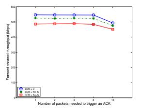
Fig. 5. Forward channel throughputs for different acknowledgement frequency in RWBP
