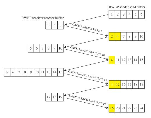
Fig. 3. Error control in RWBP. CACK : Cumulatively acknowledged; SACK : Selectively acknowledged; RE : Right edge
