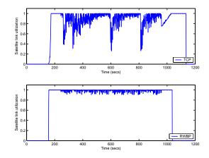
Fig. 11. Satellite link utilization for TCP and RWP with high priority UDP traffic
