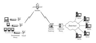
Fig. 1. Direct to user satellite networks (star topology)
