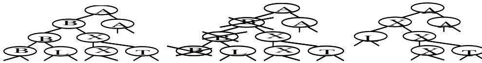
Figure 3.19. Schedule maintenance after B 's failure, when parent A = P(B) “replaces” B .
