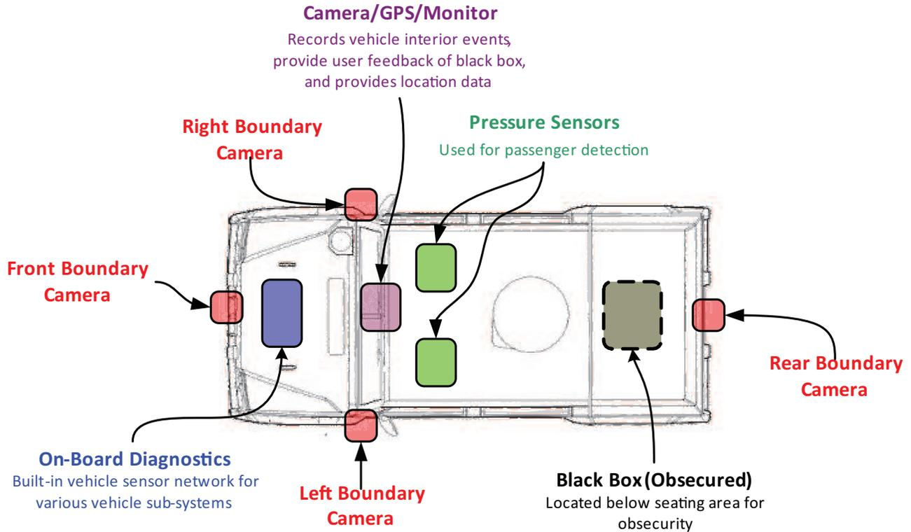
Figure 2.3: Complete Black Box system layout diagram showing the location of each subsystem
