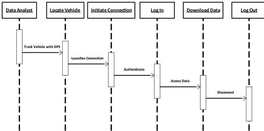
Figure 4.8: Sequence Diagram of Retrieving Data
