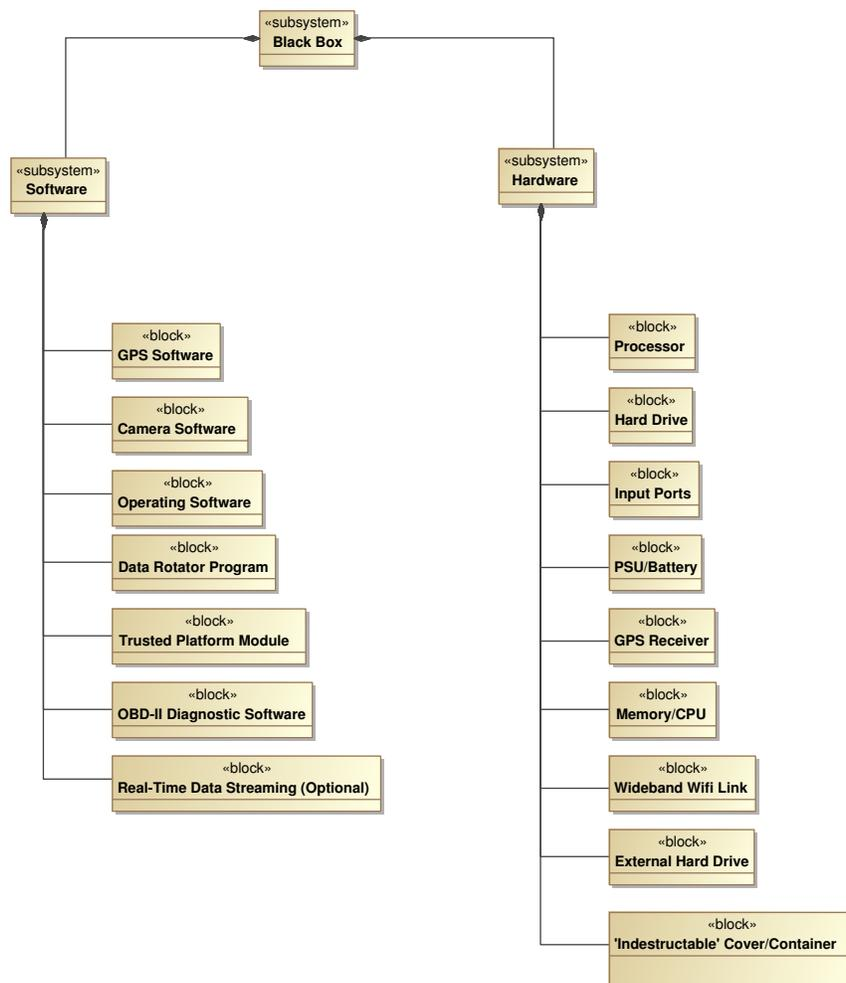
Figure 6.2: Black Box Structure Diagram
