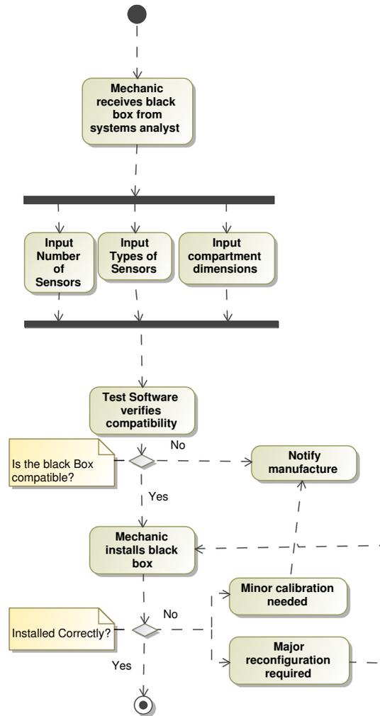
Figure 3.1: Activity Diagram for Installation and Testing
