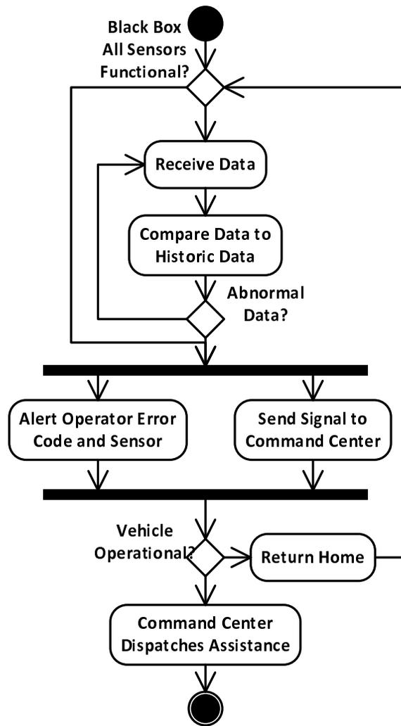
Figure 3.7: Activity Diagram for Maintenance
