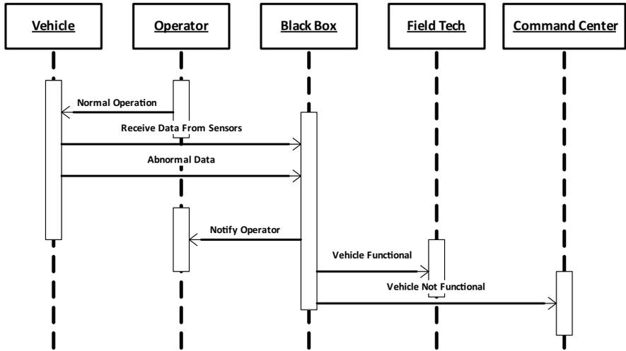
Figure 4.9: Sequence Diagram of Maintenance
