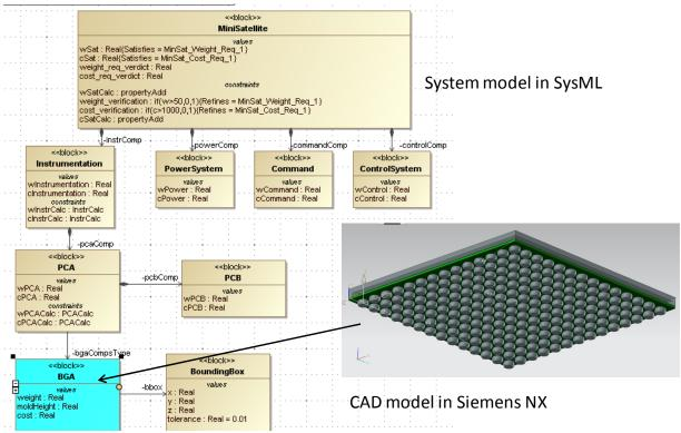
Figure 16: Mini-Satellite system model in SysML. The BGA electronic component and its CAD definition are highlighted.
