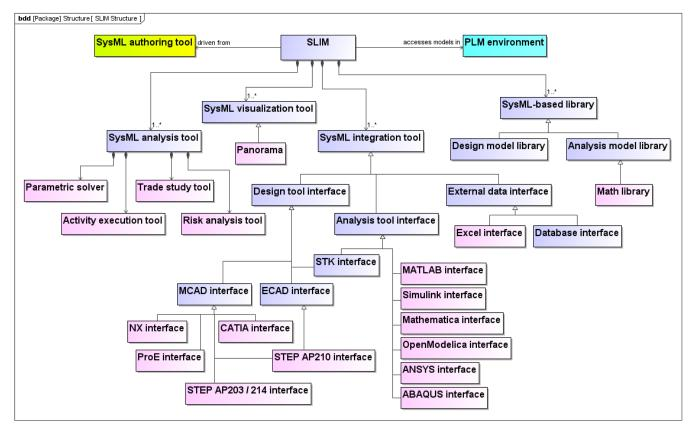
Figure 7: Conceptual decomposition of the SLIM framework
