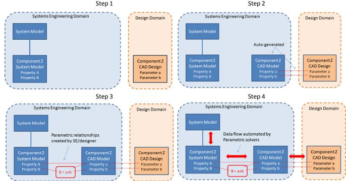
*Figure 15: SysML–Design (MCAD/ECAD, STK) integration capability – end-user steps*
