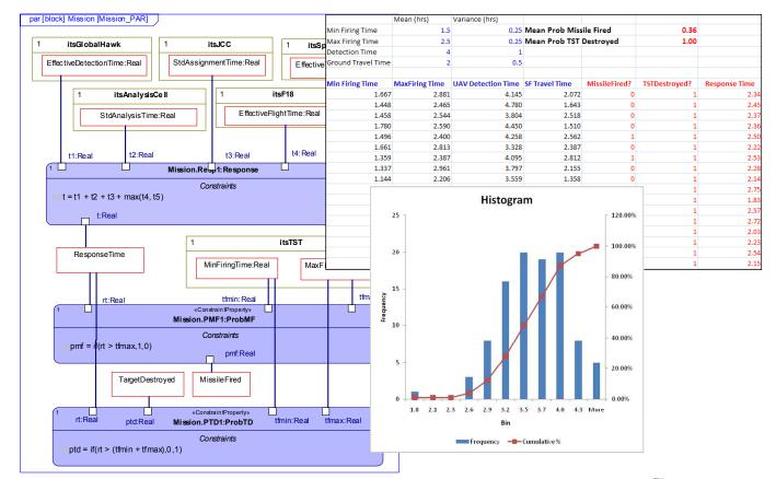
*Figure 12: Computing success probabilities & response times for military operations using Melody*<sup>™</sup> *for Rhapsody*
