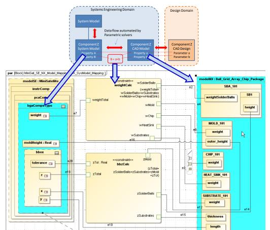
Figure 17: Parametric relationships between the BGA component in the system model and its CAD definition.
