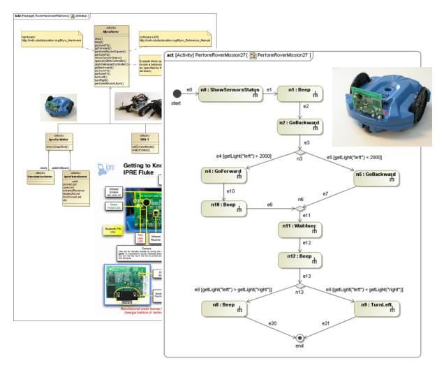
Figure 13: Activity model for driving mini-rovers using the MyroMagic plugin
