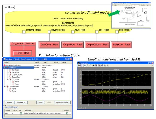
Figure 10: Parametric constraints wrapping Simulink models executed by ParaSolver (for Artisan Studio)
