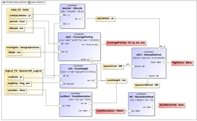
Figure 8: SysML parametric model for computing coverage, scan resolution, and flight cost of the FireSat, and for verifying resolution requirement
