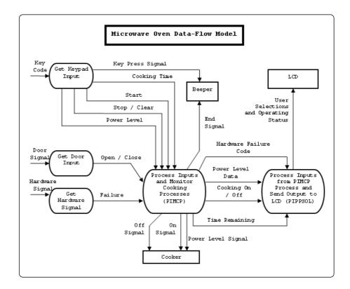
Figure 15.2. Data flow diagram for operation of a microwave oven.
