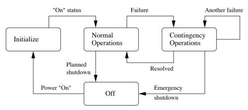
Figure 15.4. State machine model for behavior of a spacecraft computer.
