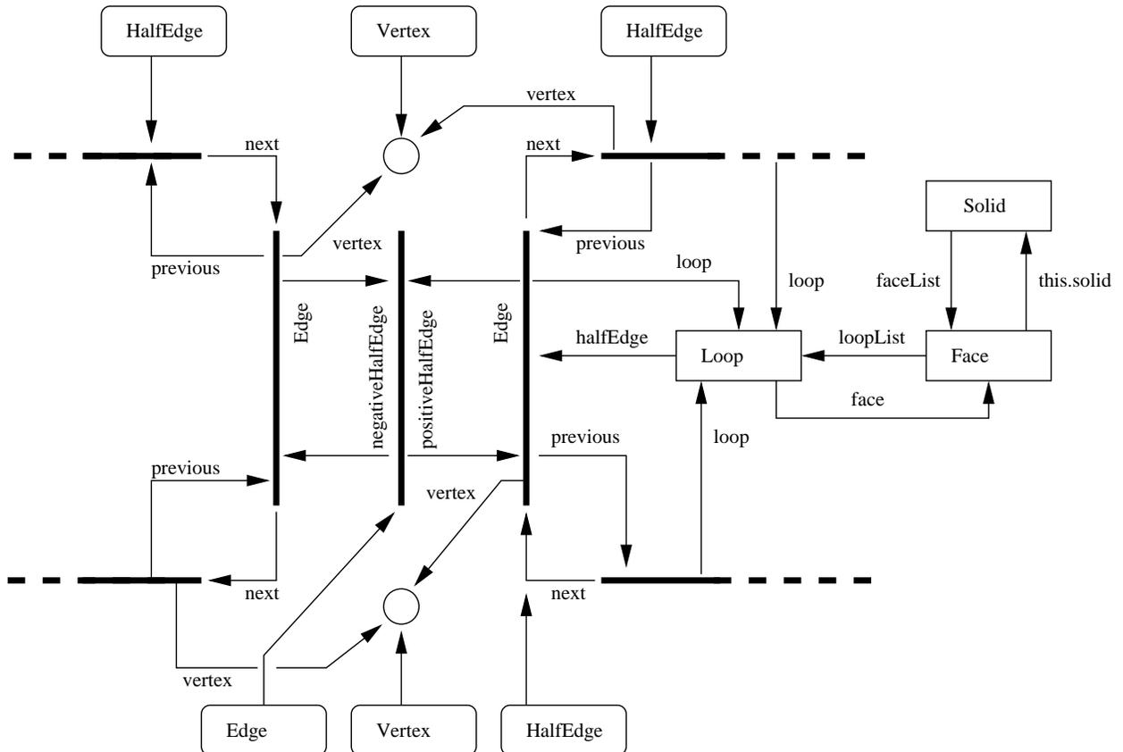
**Figure 14.7.** Schematic of relationships in the halfedge data structure. Note: Some relationships have been omitted for clarity.
