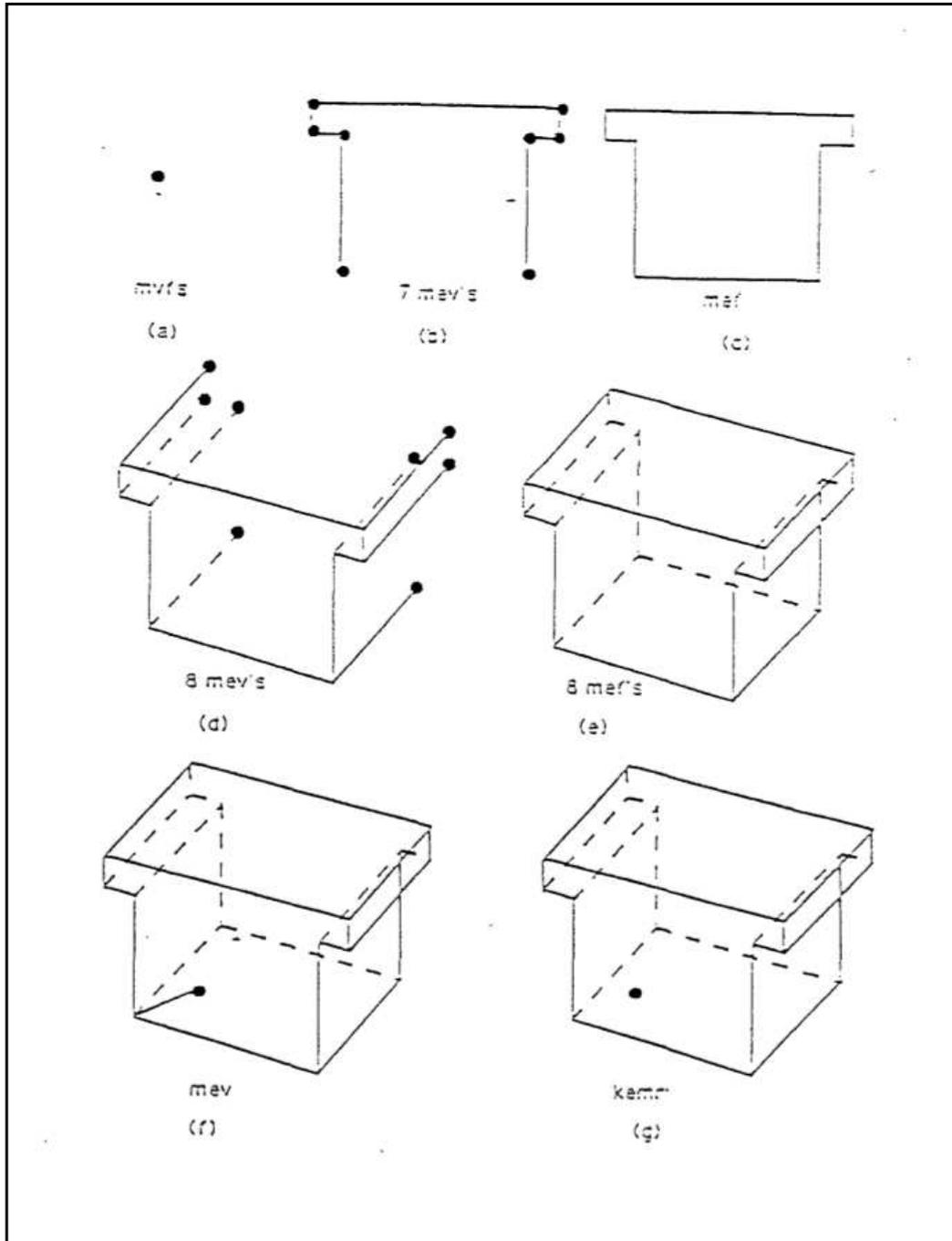
**Figure 14.5.** Using Euler operations for the step-by-step assembly of a TBeam.
