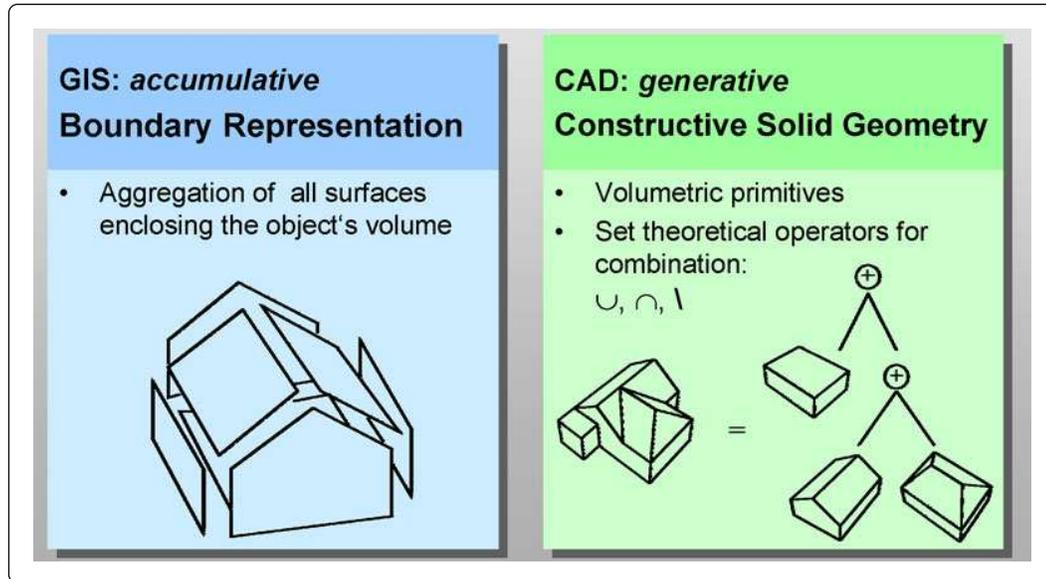
**Figure 14.2.** Boundary and constructive solid geometry (CSG) approaches to geometric modeling.
