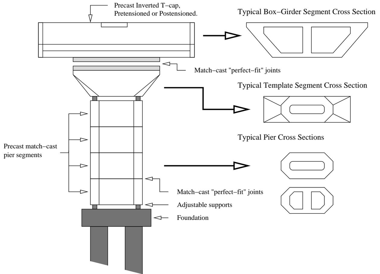
**Figure 14.1.** Elements of a precast bridge pier (Adapted from Billington [5]).
