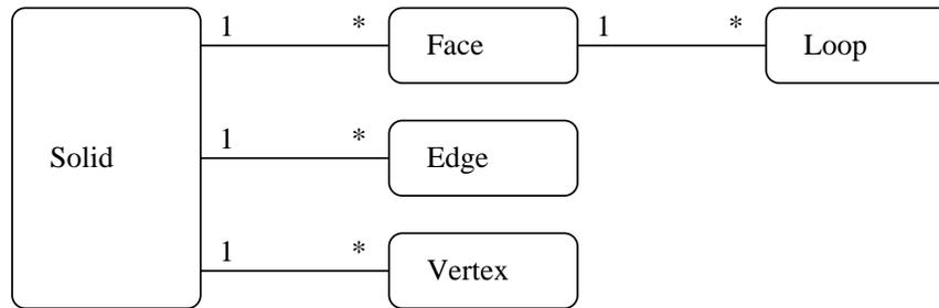
**Figure 14.8.** UML schematic of the solid data structure.
