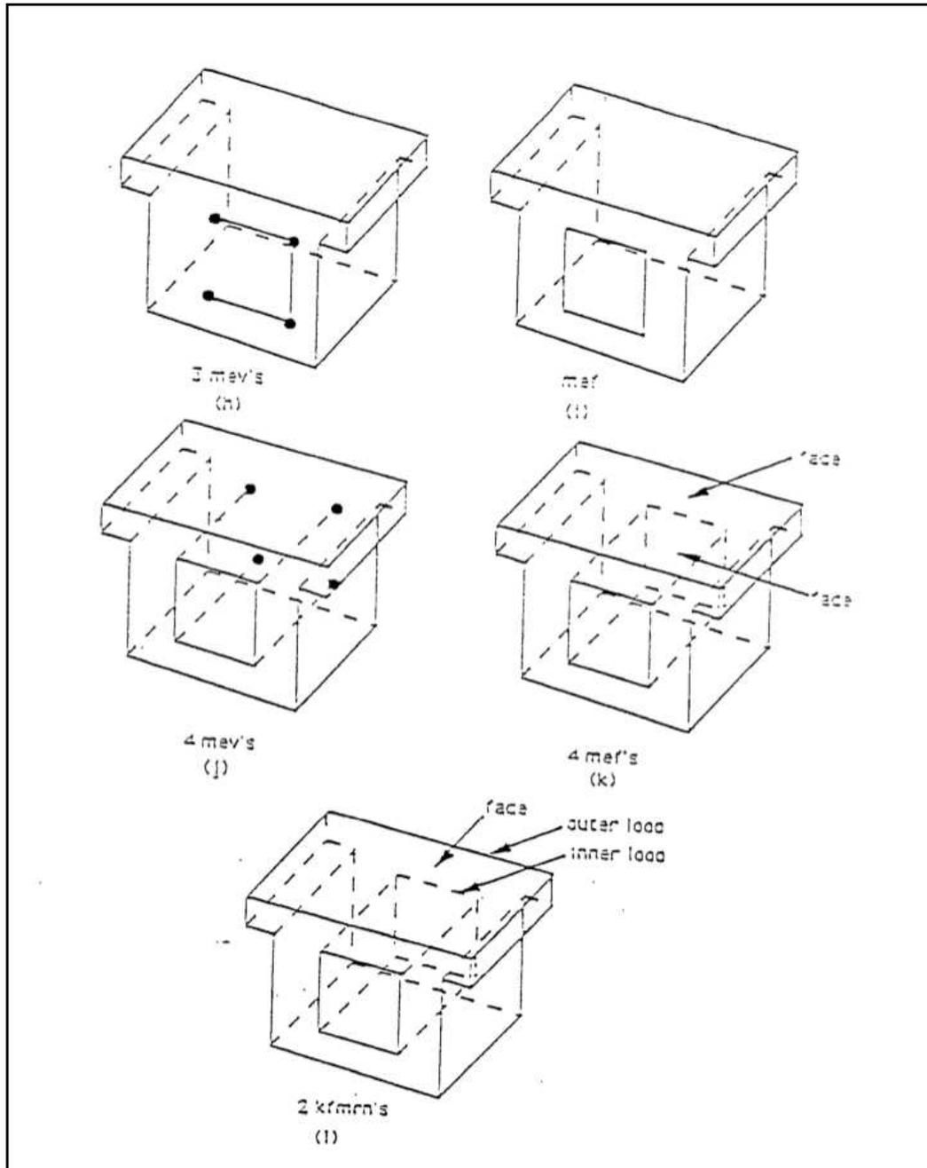
**Figure 14.6.** Using Euler operations for the step-by-step assembly of a TBeam.
