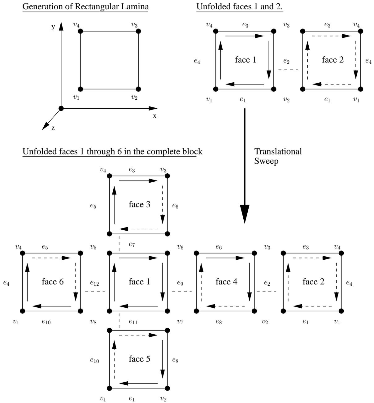
**Figure 14.11.** Schematic for systematic generation of a rectangular block. Solid oneway arrows denote a positive half edge. Negative half edges are drawn as dashed oneway arrows.
