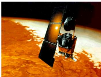
NASA's systems engineering process did not specify the [system of measurement](#). One of the development teams used Imperial measurement; the other metric.
