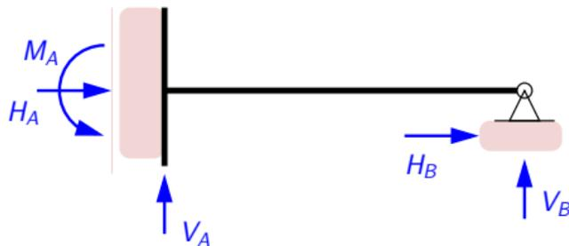
Need to release two restraints to create determinate structures,
