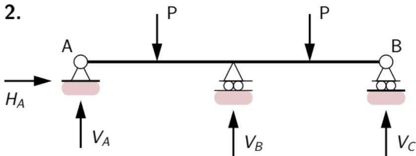
Three equations of equilibrium. Four unknowns:  $V_A$ ,  $H_A$ ,  $V_B$  and  $V_C \rightarrow 4 > 3 \rightarrow$  **statically indeterminate** to **degree 1**.
