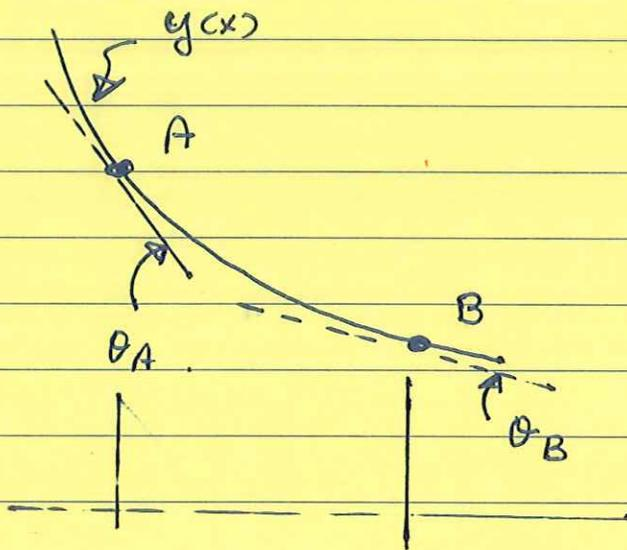
$$\frac{d^2y}{dx^2} = \phi(x) = \frac{M(x)}{EI} \quad \text{--- (C)}$$
