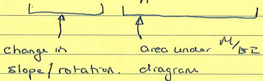
Theorem II: The distance of A to the tangent at B measured perpendicular ( $\perp$ ) to the original beam axis equals the first moment of area between A & B evaluated about A.
