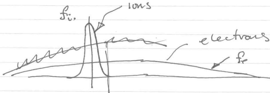
$$f_i = \frac{n_{i0}}{\left(\frac{2\pi kT_i}{m_i}\right)^{1/2}} \exp\left(-\frac{1}{2} \frac{m_i V_{te}^2}{T_i}\right)$$
