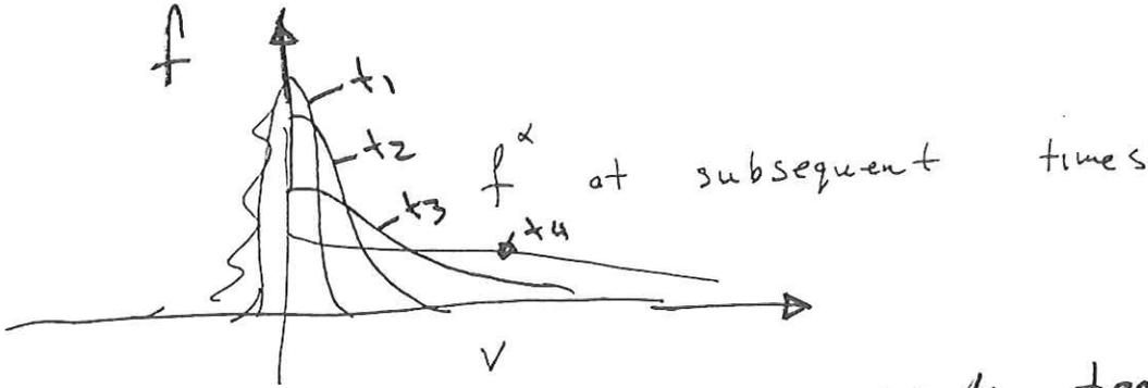
If only scattering were present temperature of type  $\alpha$  particles would increase indefinitely. When both ~~are~~ are present an equilibrium is reached  $\leftarrow$  slowing down of energy diffusion  $\leftarrow$
