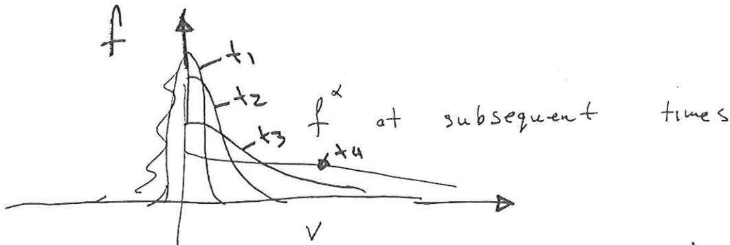
If only scattering were present temperature of type α particles would increase indefinitely. When both ~~are~~ are present an equilibrium is reached
